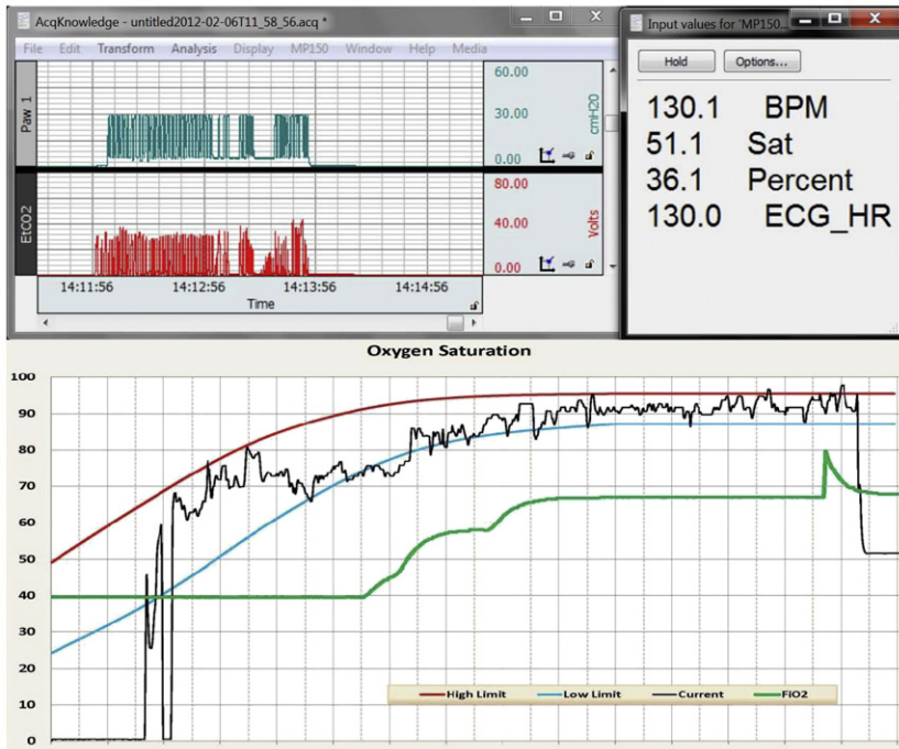
Fig. 2. Flat-screen monitor display of SaO 2 normative curves (bottom, as in TOTS), airway pressure, end tidal CO 2 graphic display (top left), ECG, pulse rate from oximeter, SpO 2 , percent inspired oxygen and ECG derived HR. Digital display (top right).
